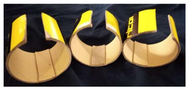
5. Arrange the rings along the other tube, so that the cut-out sections hold the slot open.
